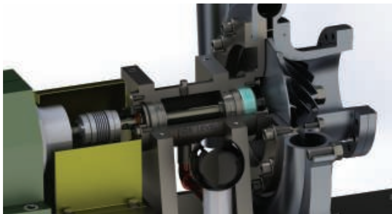
FIGURE 6. A robust compressor-design software evaluates the performance and characteristics of journal bearings, as well as many other operational considerations
