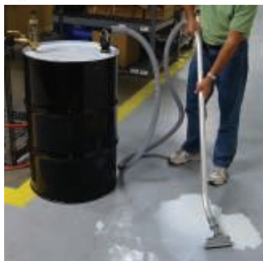
FIGURE 4. The Dual Force Vac Drum uses Vortec technology, which is a two-way, air-powered drum pump that can fill or discharge a 55-gal drum in 2 minutes. It can handle viscous liquids to 1,500 cP, as well as chips and particulate, making it suitable for cleaning solvents, hydraulic oil, liquid spills, liquid transfers and more
