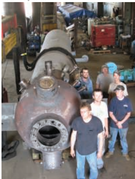
FIGURE 2. The term "shell-and-tube heat exchanger" incorporates a wide range of equipment variations, such as this model in the shop
