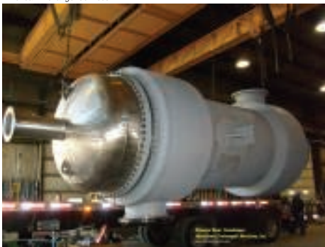
FIGURE 3. Finite element analysis was used for the design of the flexible shell element of this large exchanger
