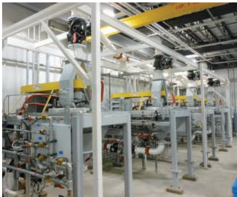
FIGURE 4. In recent years, pin mills, such as this one milling trona, have become competitive with air-swept classifying mills on performance, but also can yield reduced capital, energy and operating costs
